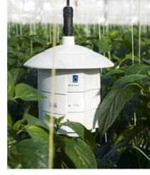
PHOTO: To make better adjustments and achieve the highest yield, climate sensors can measure temperature, relative air humidity and CO<sub>2</sub>
