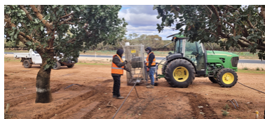
Successful recoiling of old 19-millimetre poly using the Netafim Recoil machine.
