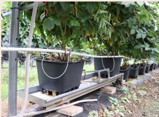
A Groscale installed amongst Aman Lehl's vines enables monitoring of plant water consumption without removing the pot from the row.
