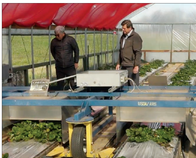
Fumiomi Takeda (left) and Wojciech Janisiewicz with a prototype machine capable of delivering low doses of UV-light to strawberry plants.
