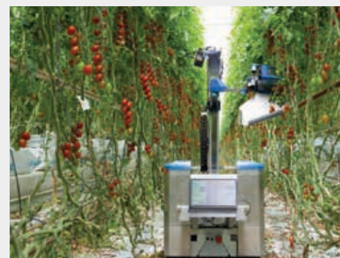
The inaho robot at work harvesting snacking tomatoes in a Dutch glasshouse.
